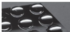
Figure 1. Photograph of a chip with immobilized DNA and filler after washing and inverting the chip. DNA-bearing spots retain the aqueous solution preferentially over the surrounding areas. During hybridization, a cover slip may be used to ensure contact between all spots and the solution.
